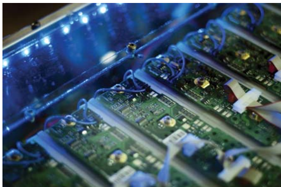
Battery management system
